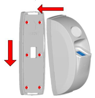
Once the head unit is attached on to the backplate, push against the head unit until you hear the security clips click into place.
