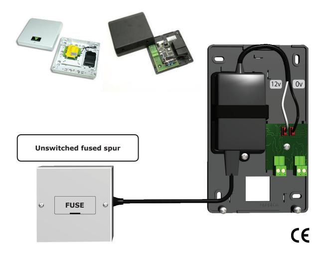
The figure 8 power lead provided is pre-stripped at one end for connection to a fused spur.
