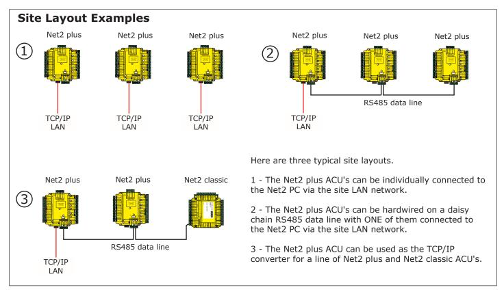
The TCP/IP interface allows an RS485 data line to be controlled by the Net2 Server running across a LAN network.
