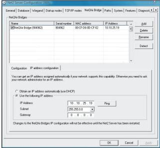
Click on **Detect** and the MAC address of the device(s) will appear in the table. You must then use the "IP address configuration" tab to manually assign the IP address, subnet mask and gateway.
