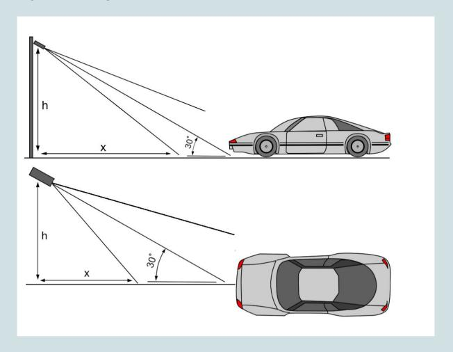
You can measure all of the needed geometrical lengths using a Pythagorean equation. But it is sometimes hard to measure the angles properly.
