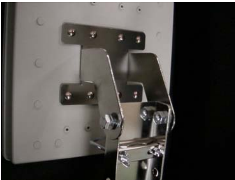
(3) Assemble bracket to mounting plate by using 2 hex bolts/nuts
