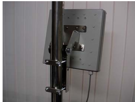
(4) Install mounting bracket to the pole then adjust the angle of the reader
