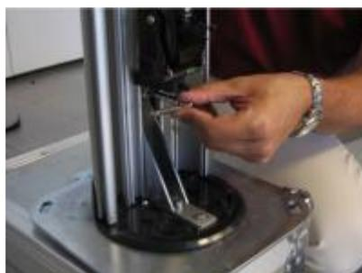
On the top of each column there are two tamper switches. The one on the side provides information about the top cover removal. The one on the centre, on the other hand, provides information regarding the top cover pushing and it is suitable in order to detect climbing attempts.
