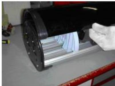
Place the bottom lid of the column on the base, place the column into the proper plug and after placing the "L" locking racket, tighten them up by using the provided screws.
