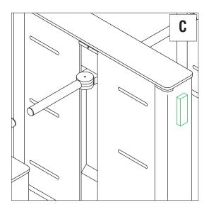
**Option C**Mounted externally directly onto square end.
